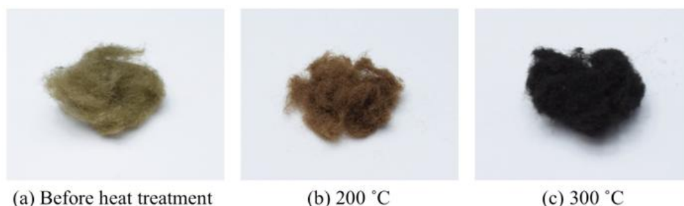
Figure 5. Effect of heat treatment of polymer-coated cottons. The samples (b) and (c) were prepared by heat treatment for 12h at 200 °C and 300 °C, respectively, under N 2 atmosphere.
